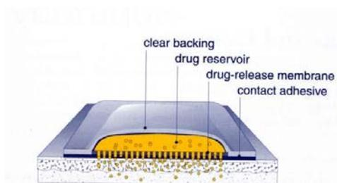
Figure 1: Deponit patch schematic
