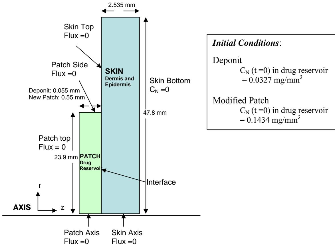
Figure 1: Schematic of Deponit patch and our modified patch
