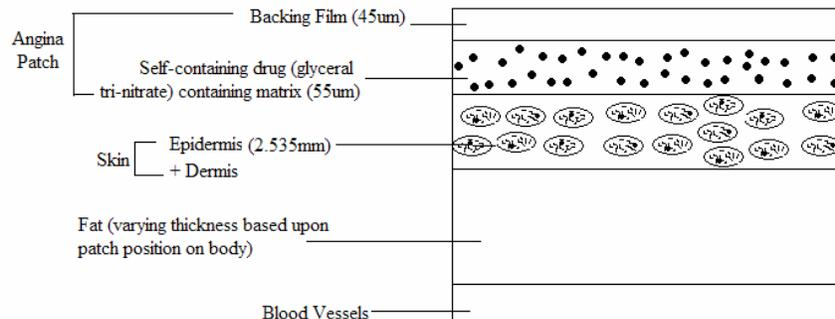
Figure 2: Diagram showing the dimensions of the three layers of the patch and skin
