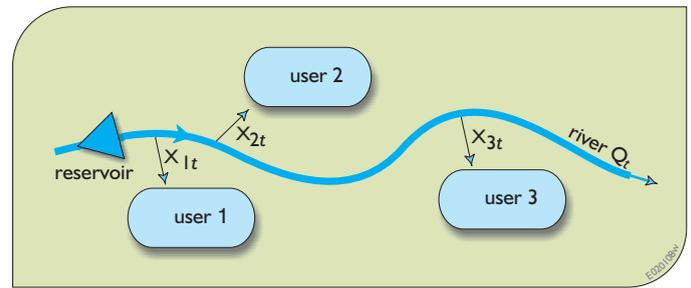
Figure 3.2. Reservoir-water allocation system to be simulated.
